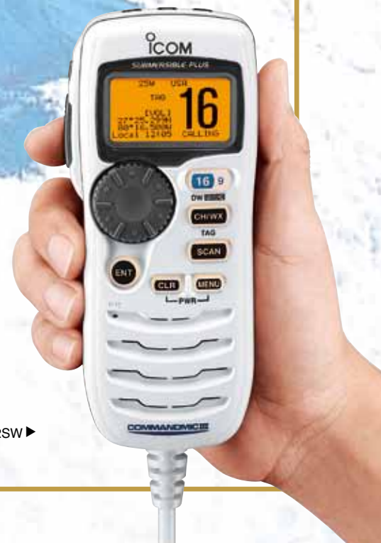
Backlit keypad and Jog dial "Distress" button on the back of the unit
